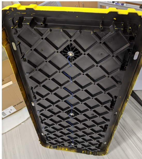
Fig. 45. Underside of UWOC tank lid with LEDs
